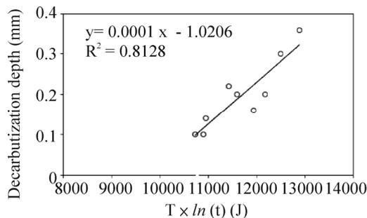
**Fig. 4.** The regression analysis of decarburization depth and  $T \times \ln(t)$ .
