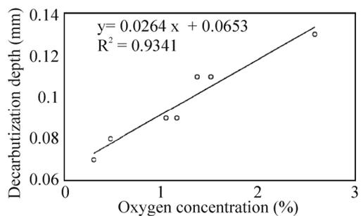
**Fig. 6.** The regression analysis of decarburization depth and oxygen content.
