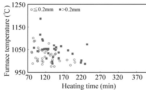
**Fig. 5.** Scatter plot of furnace temperature and heating time for decarburization depth.
