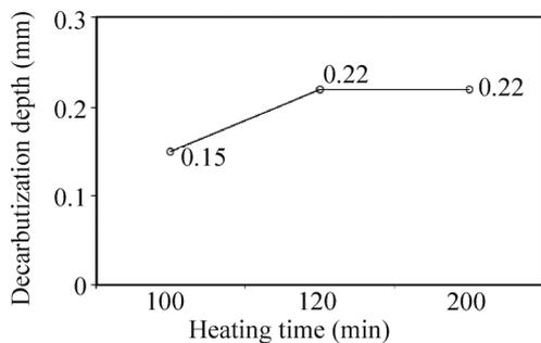
**Fig. 3.** Main factor response diagram of decarburization depth and heating time.
