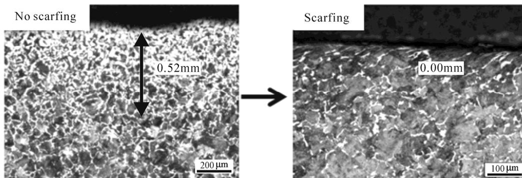
Fig.1. The change of decarburization depth in OM morphology for billet through the scarfing process.
